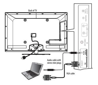
3 Connect an audio cable with stereo mini plugs to the **PC/DVI AUDIO IN** jack on the side of your TV and to the **LINE OUT** or **AUDIO OUT** jack on the computer.
